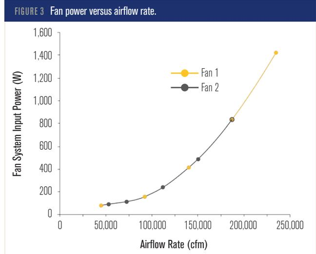
fundamental issue with rating or comparing fans based only on efficacy and using percentage of maximum speed as a basis for the comparison. A simple way to improve fan efficacy is to simply decrease the maximum speed of the fan.
